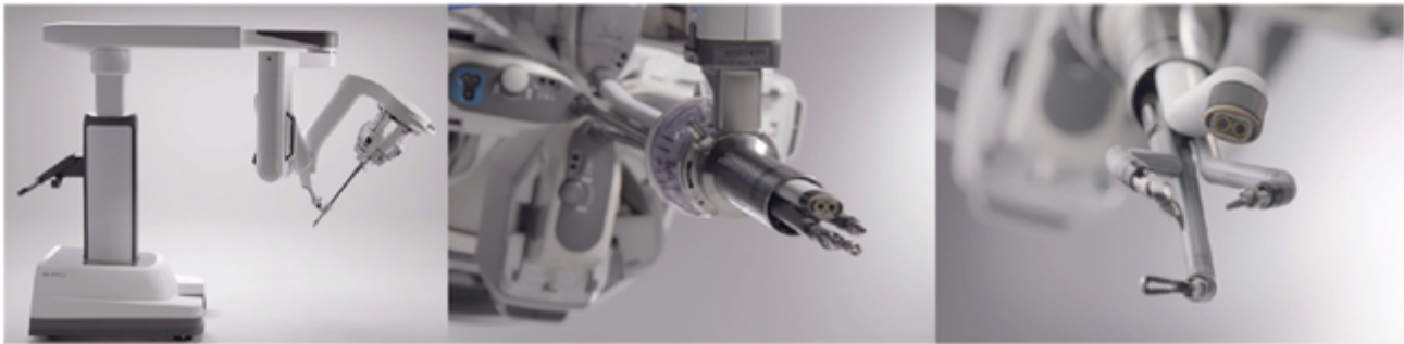
그림 1. Robotic single-incision surgery module designed by Intuitive Surgical, ©2019 Intuitive Surgical, Inc [Int J Med Robot. 2020;16(3):e2091] 6
