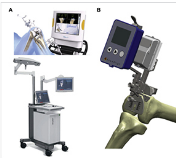
그림 1. (A) Typical large console computer navigation systems; (B) OrthAlign handheld computer navigation system
